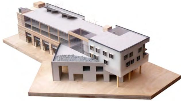
*Above & Below* The physical form and internal spatial qualities of the building were developed in a series of large scale physical models.
